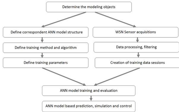
Fig. 1. The WSN data based ANN modeling procedure.
