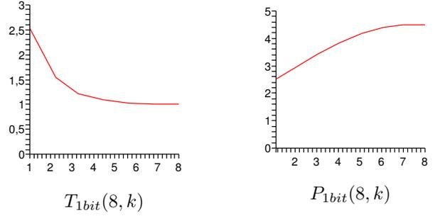
Fig. 2. Power and time consumption for transmitting each data bit in a 8 wire bus using at most  $k$  wires at each clock cycle
