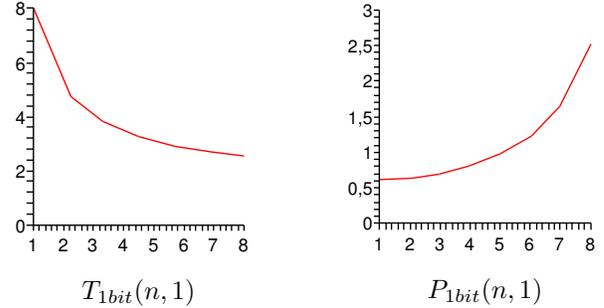
Fig. 3. Power and time consumption for transmitting each data bit in a  $n$  wire bus using at most 1 wire at each clock cycle
